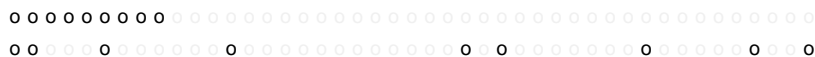
Figure 2.: On top is the output pupil of a fully redundant configuration. On the bottom is the non-redundant configuration used in the prototype FIRST instrument.
