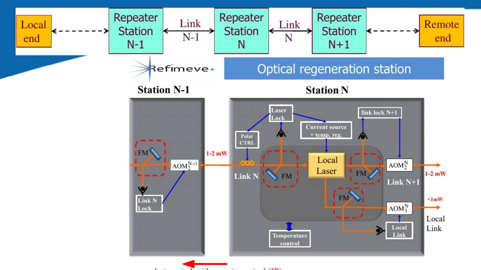
Here the signal is perfect Receive from station N 2 times distorted signal, compensates it in order To be perfect at N
