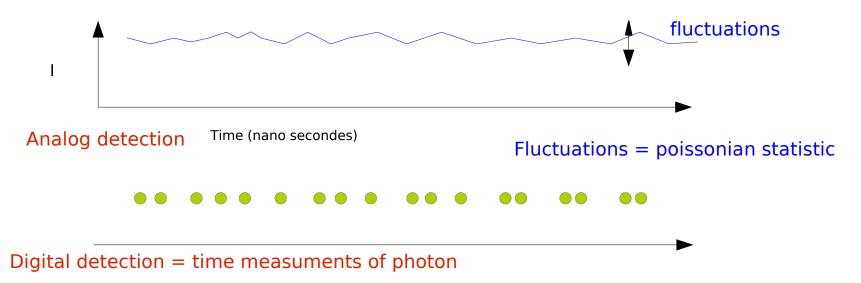
We can consider detector analog signal as a flow of photo-events
