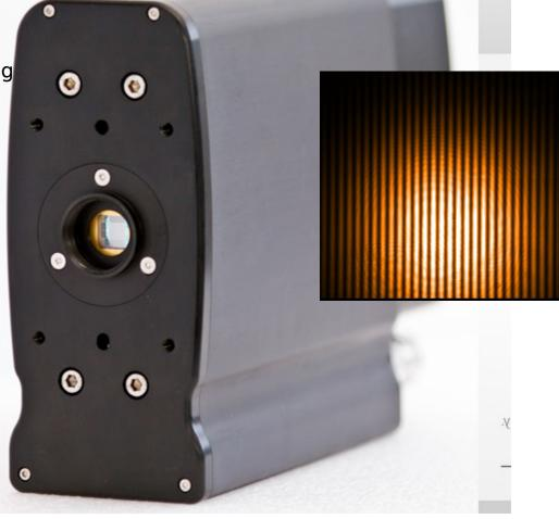
Two optical fibers are mounted on  $127\mu m$  Vgroove directly placed in front of CCD camera some fringes are due to glass window
