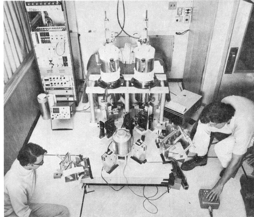
*Mid-IR ( $10\ \mu\text{m}$ ) interferometry using heterodyne detection. 5.5 m baseline separation between auxiliary siderostats*
