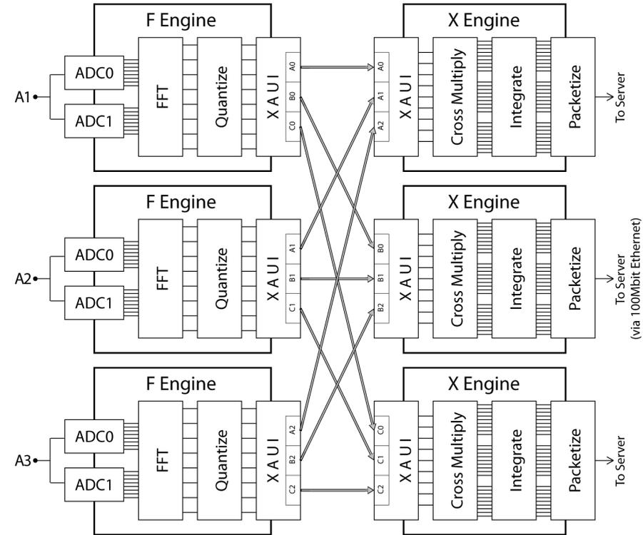
6 Gsamp/sec using interleaved ADCs
