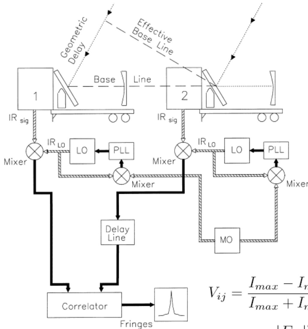
Heterodyne detection using CO<sub>2</sub> lasers as local oscillators
