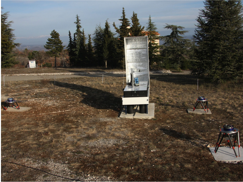
Figure 3.: View of the three primary segments: the mirrors are disposed on rigid carbon legs, and manually adjustable in tip-tilt and piston (This pictures has already been published in Le Coroller et al. 2012)
