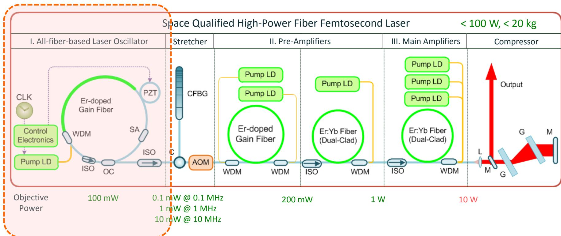
*Master oscillator determines <sup>1</sup>pulse duration, <sup>2</sup>repetition rate, <sup>3</sup>spectral bandwidth, <sup>4</sup>power stability and so on*
